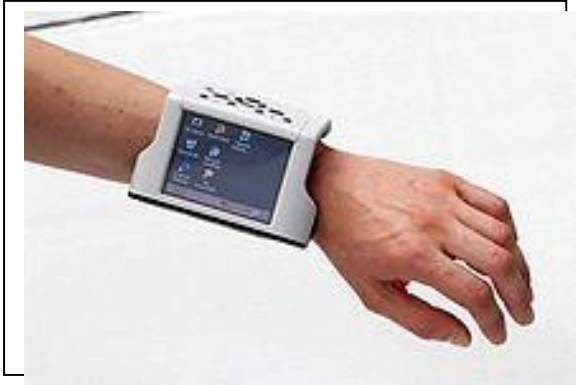
Figure 2: Image of the ZYPAD wrist wearable computer from Arcrom Control Systems [3][9][13]
